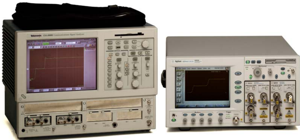
Figure 2-1 TDR-based Physical Layer Test System Hardware: Tektronix CSA8000 (left) and Keysight 86100A/B/C DCA (right)
